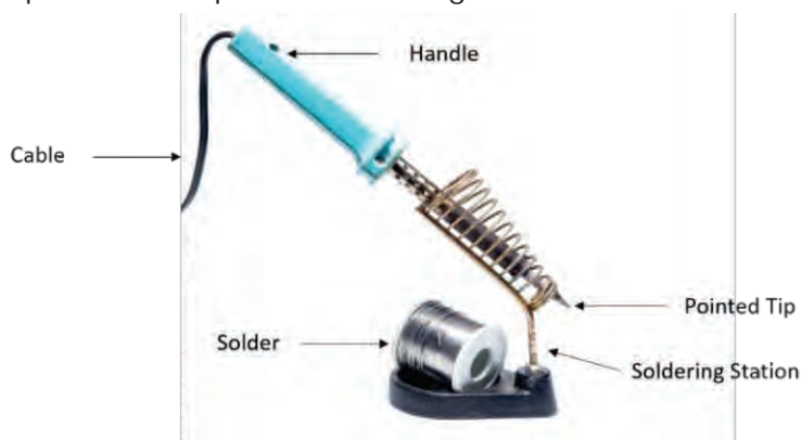
Fig 1.3.3: Parts of soldering iron
